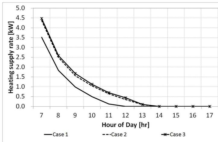
**Figure 4.** Hourly supplied heat by the system in the middle floor west zone (Jan. 14<sup>th</sup>) (Lee et al. 2012)
