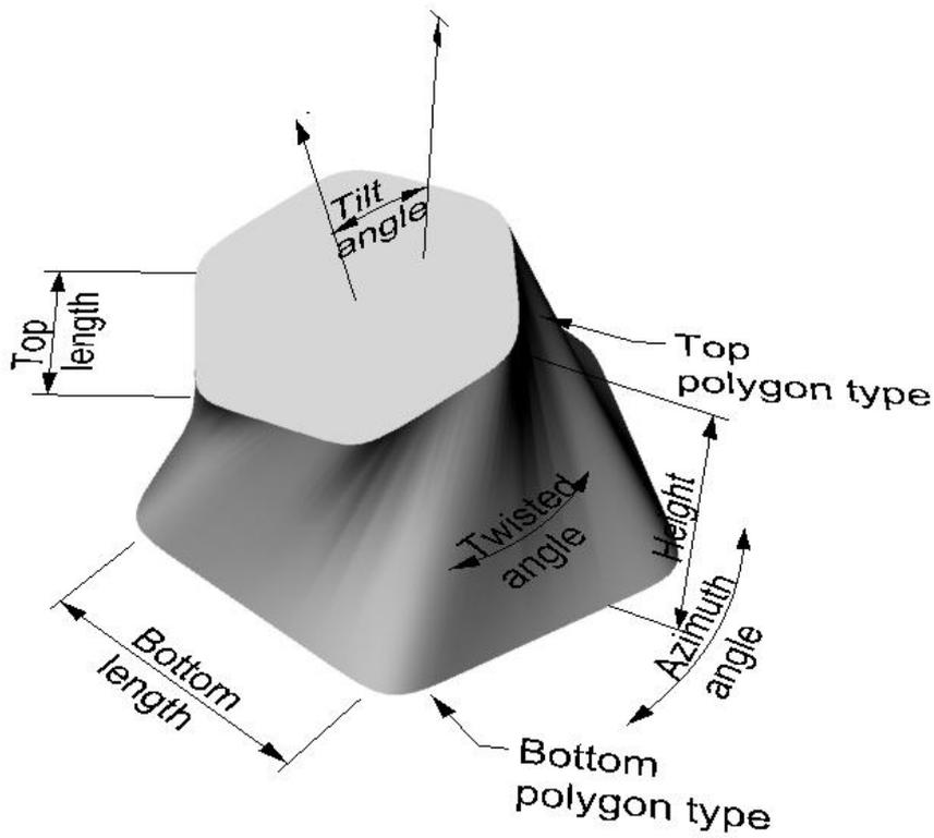
**Figure 1.** Design parameters of the reference building
