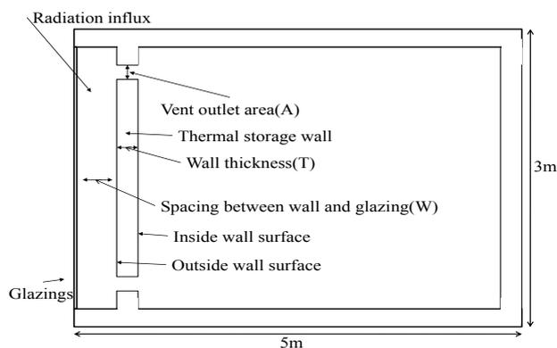
**Figure 1.** Cross-section drawing of the subject space
