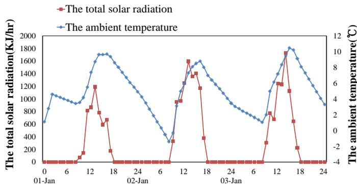
**Figure 2** Total solar radiation and ambient temperature of representative date
