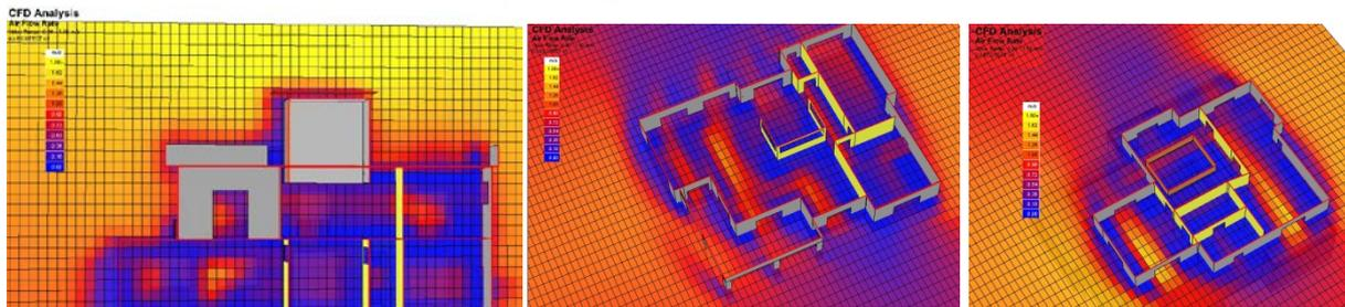
**Figure 7.** Airflow through the wind catcher and windows (XZ axis section); airflows in the ground and first floor
