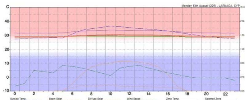
**Figure 8.** Hourly temperature of the first floor plan after applying new materials
