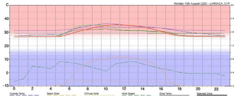
**Figure 9.** Hourly temperature of first floor plan after applying the wind catcher and insulation
