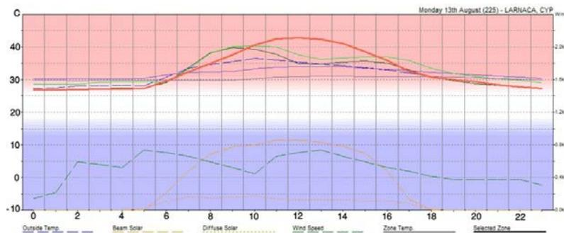
**Figure 6.** Hourly temperature of first floor plan after applying the wind catcher
