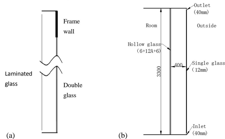
**Figure 1.** Sketch of the DSF window. (a) A sketch of model 1, and (b) A sketch of model 2 and model 3.
