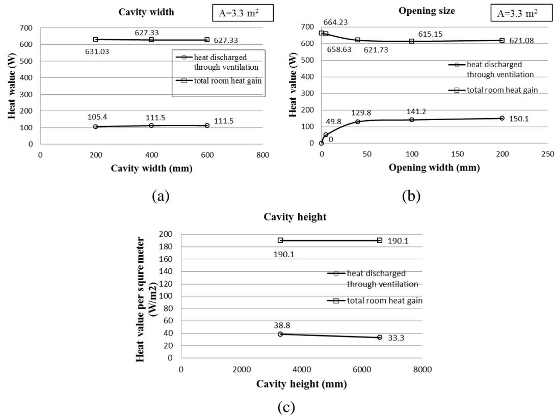
**Figure 3.** Influences of three parameters on thermal performance of the DSF.
