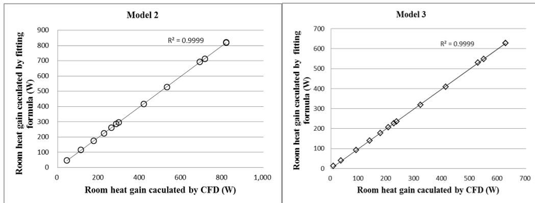
**Figure 2.** CFD simulation results compared with the linear model. Hollow points represent the value of the room heat gain, while lines represent the line  $y=x$ .
