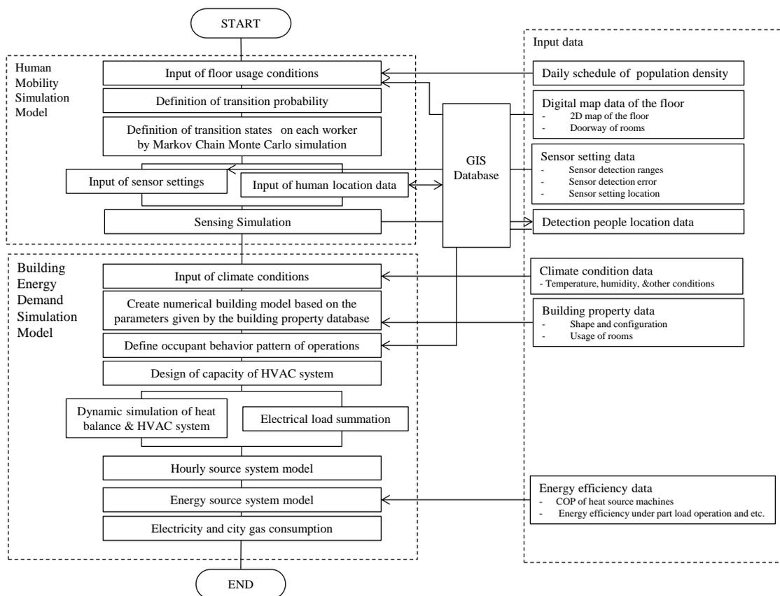
**Figure 1. Overall flowchart of simulation model**
