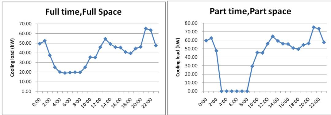
**Figure 5** Cooling load curve of single residential building (typical day, 12/8/2011)
