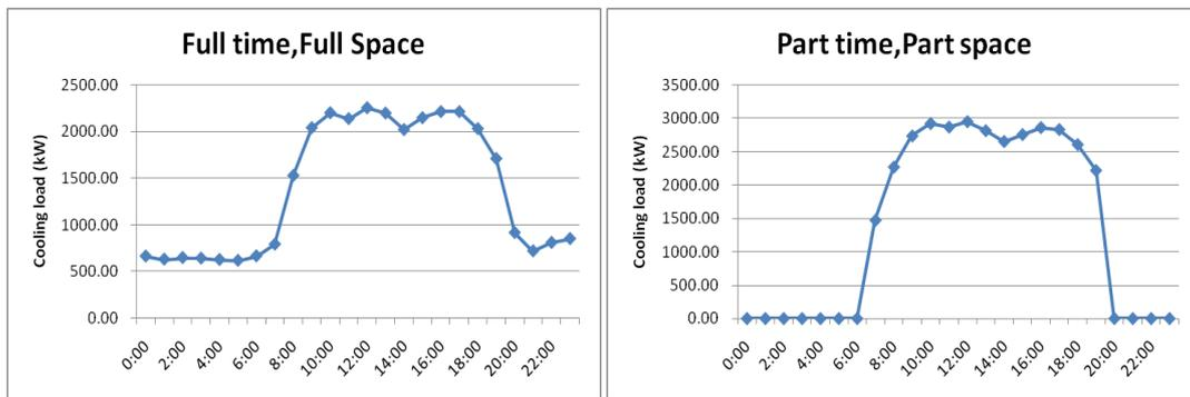
**Figure 6** Cooling load curve of single office building (typical day, 12/8/2011)
