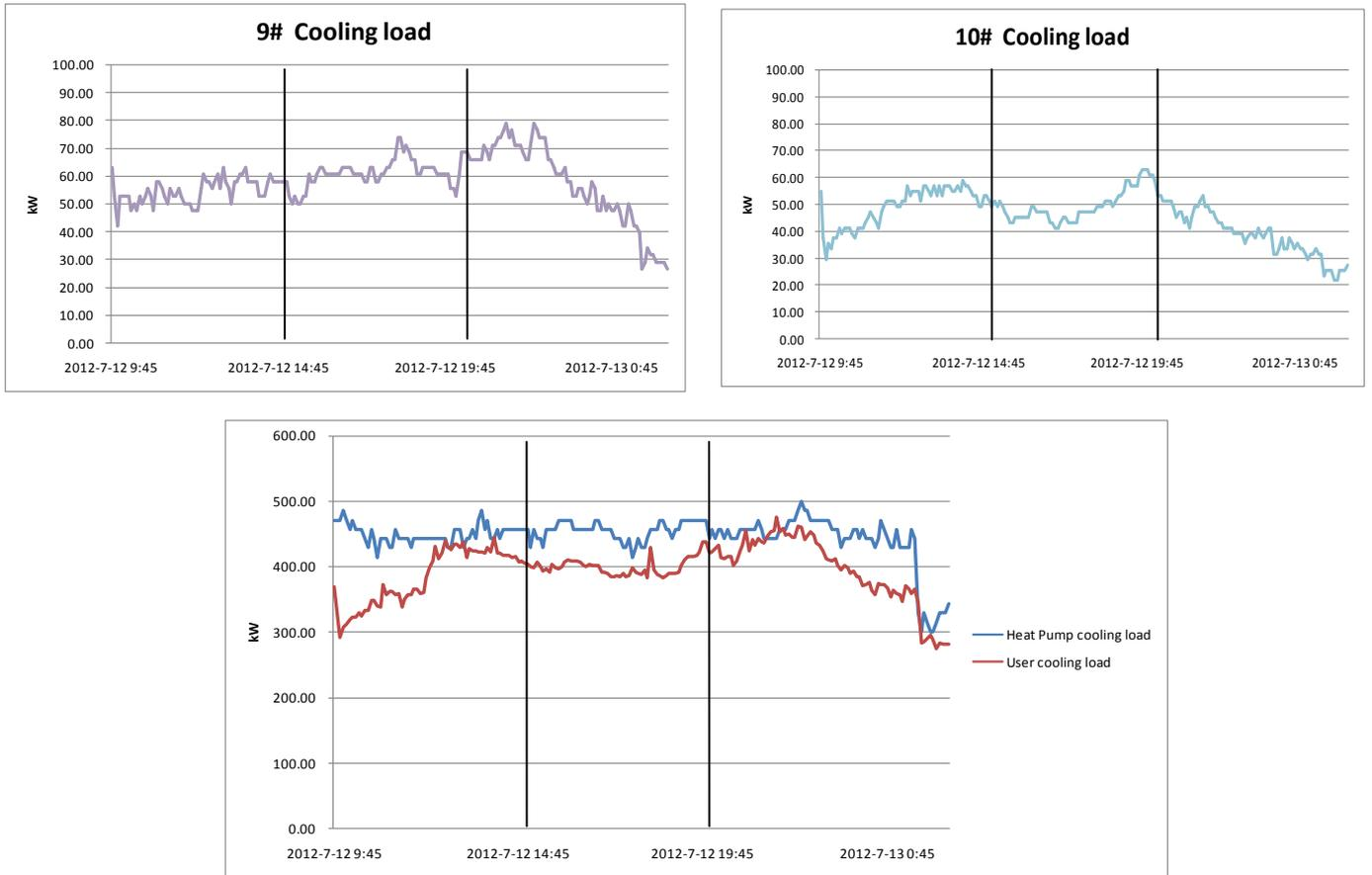
**Figure 3** Typical residential building and system cooling load curve of JY
