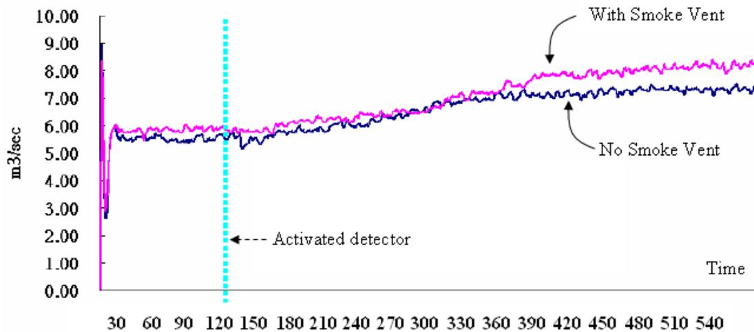
**Figure 5.** Flow volume of the ventilation tower
