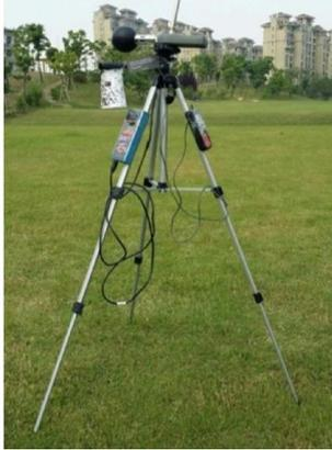
**Figure 2.** Home-made micro weather station diagram
