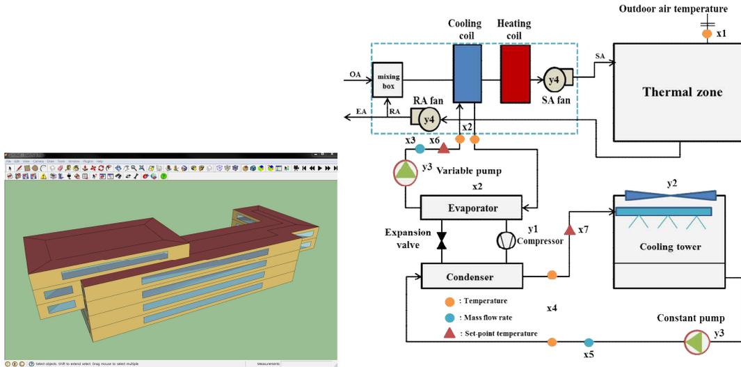
**Figure 1.** EnergyPlus model and dataset collected from the chiller system (noted as  $x^*$  and  $y^*$ )
