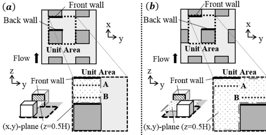
Fig. 5 Schematics of data sampling positions for (a) SQ and (b) ST. The snapshots of wall pressure distribution are extracted at front and back walls. The snapshots of flow structures are obtained at  $(x, y)$ -planes at the height of  $1.5H$  (in unit area),  $1H$ ,  $0.5H$ , and  $0.16H$ , and at  $(y, z)$ -planes: A and B separated by  $0.22H$  from front and back walls, respectively.
