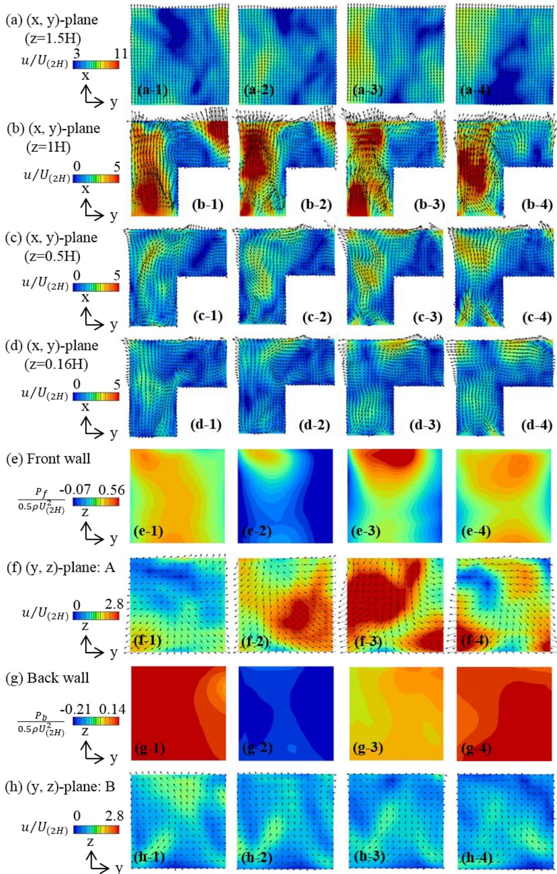
Fig. 7 Instantaneous distributions of velocity and pressure for ST in planes shown in Fig. 5. The number indicates the sampling time: from 1 to 4 for 105s, 105.02s, 105.04s, and 105.06s, respectively.
