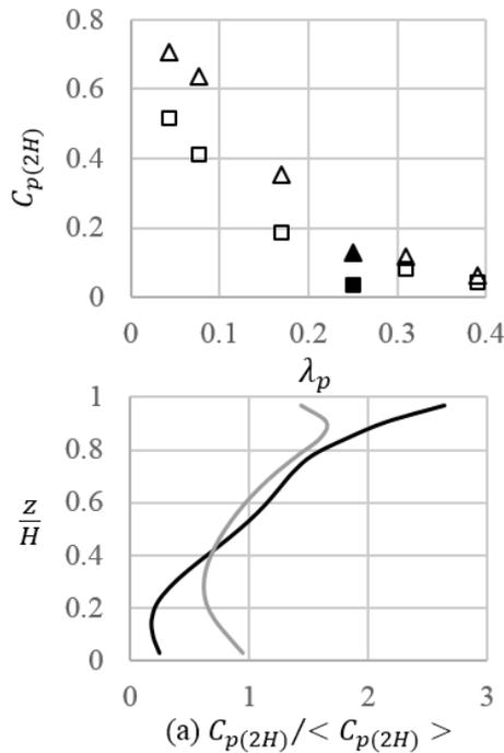
Fig. 2 Wind pressure coefficient:  $C_p$  defined by mean velocity at  $z=2H$  for different packing densities.  $\blacksquare$ : SQ.  $\blacktriangle$ : ST.  $\square$ : SQ1 and  $\triangle$ : ST1 (Zaki et al., 2012).
