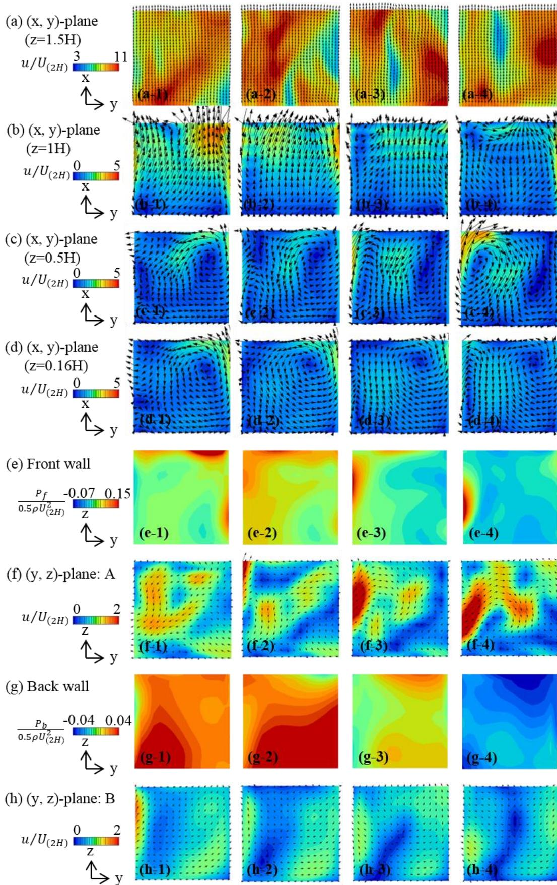
Fig. 6 Instantaneous distributions of velocity and pressure for SQ in planes shown in Fig. 5. The number indicates the sampling time: from 1 to 4 for 105s, 105.02s, 105.04s, and 105.06s, respectively.
