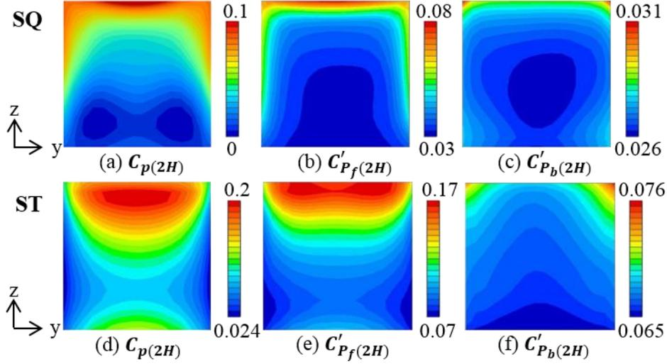
Fig. 4 Surface distributions of (a) wind pressure coefficient and fluctuating wind pressure coefficient on (b) front and (c) back surface defined by the reference velocity at  $z=2H$  for SQ. (d), (e) and (f) are the same as (a), (b) and (c), but for ST.
