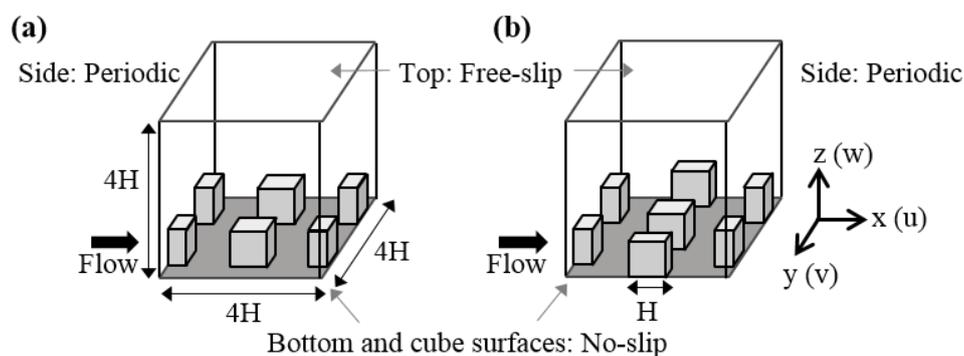
Fig. 1 Schematics of computational domain. (a) Square array: SQ (b) Staggered array: ST
