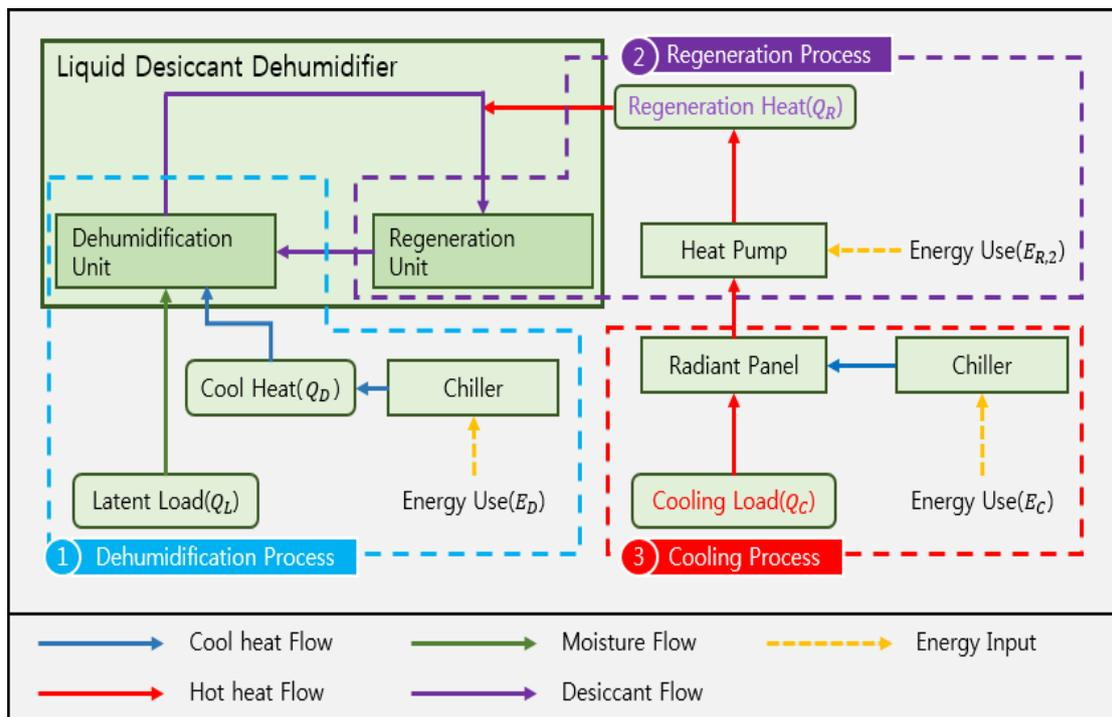
Figure 2. Schematic diagram of Method 2
