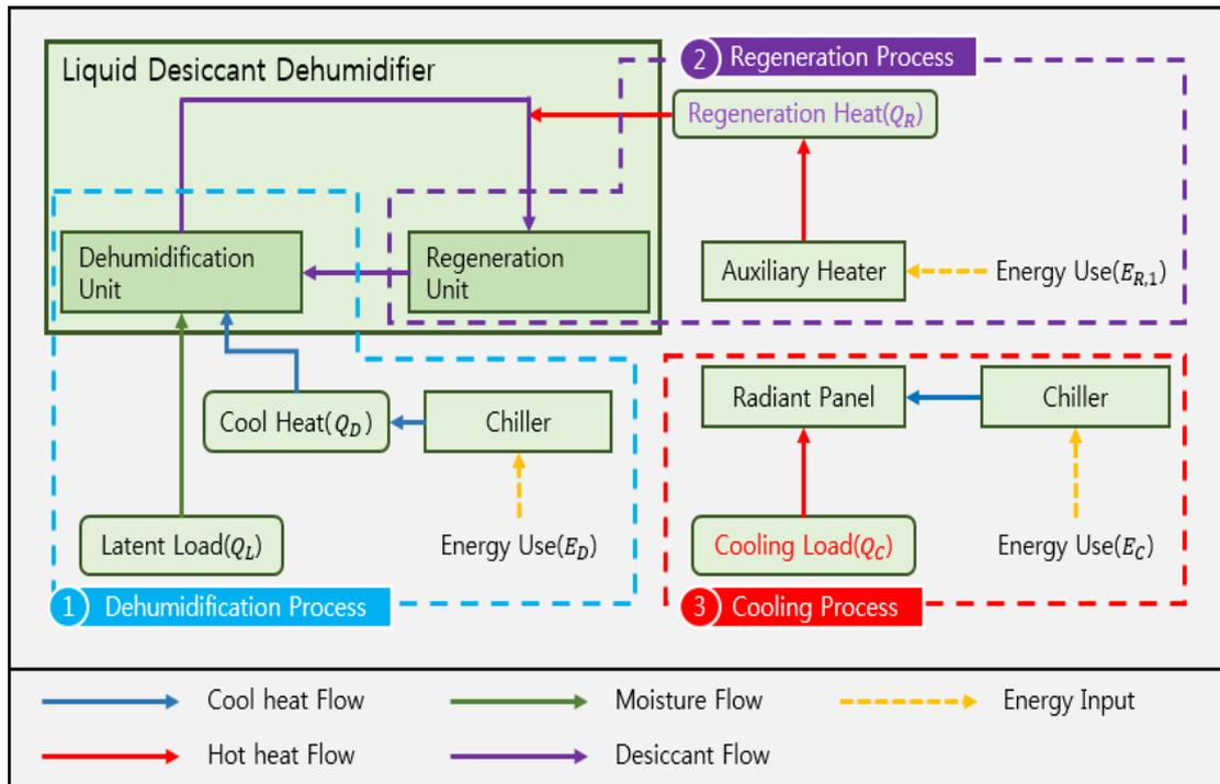
Figure 1. Schematic diagram of Method 1
