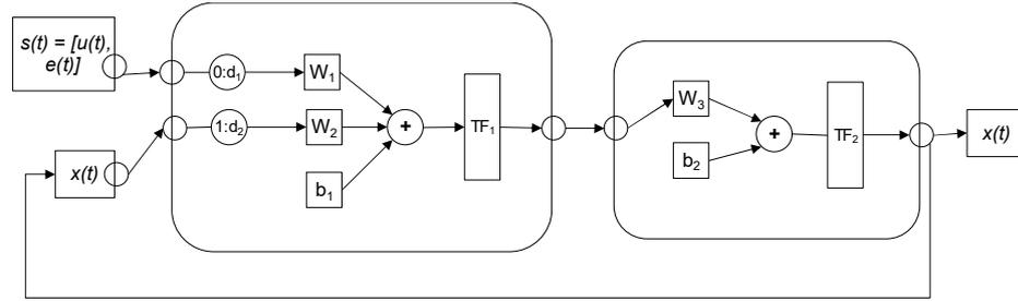
**Figure 1.** NARX model for thermal behavior of building
