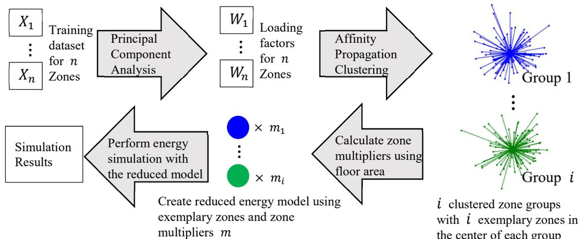
**Figure 1.** Procedures of the proposed model reduction method
