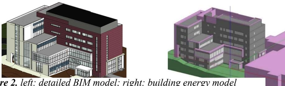
*Figure 2. left: detailed BIM model; right: building energy model*
