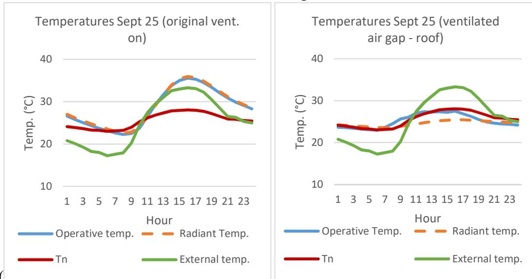
**Figure 6).** It is observed that in the building of the original features, the indoor temperatures were higher than the outdoor temperatures. The strategy of ventilated air gap of the roof with polystyrene and zinc presented the most similar curve to the neutral temperature and the radiant temperature values were lower during the hottest hours.
