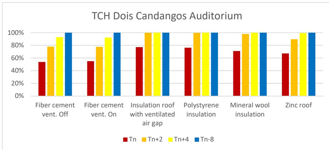
**Figure 4.** TCH analysis of roof material without influence of lighting system
