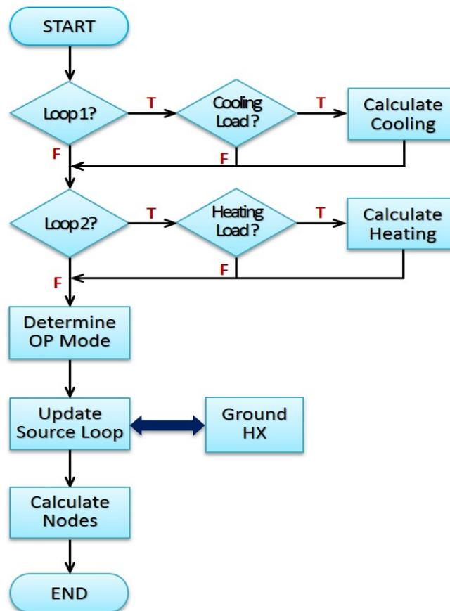
**Figure 2.** The modeling process for a CGSHP system
