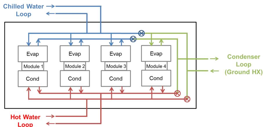
**Figure 1.** An example diagram of a central heat pump system with three chiller-heaters in heat recovery mode and one chiller-heater in heating-only mode
