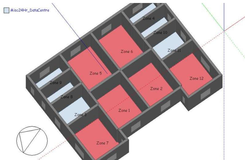
**Figure 3.** Top thermal zones. Source: DesignBuilder version 2.2.5.004.
