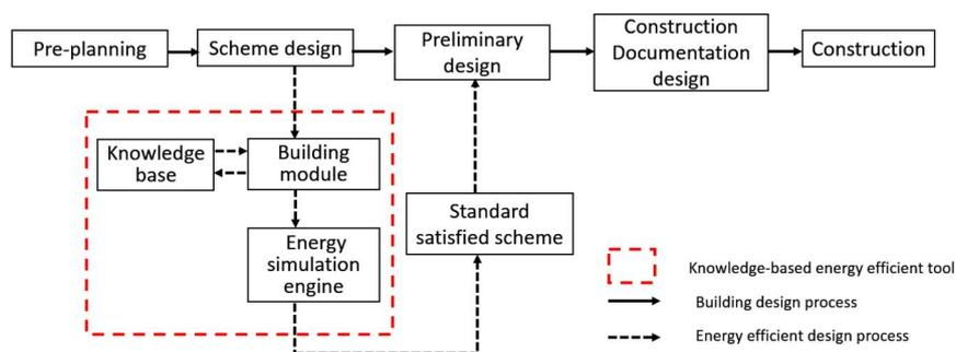
*Fig. 2. Knowledge-based energy efficiency design process*
