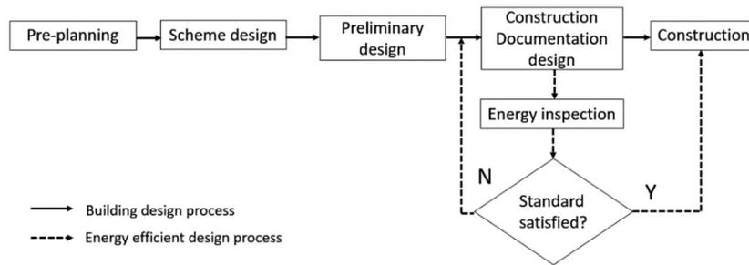
*Fig. 1. Current energy efficiency design process in China*
