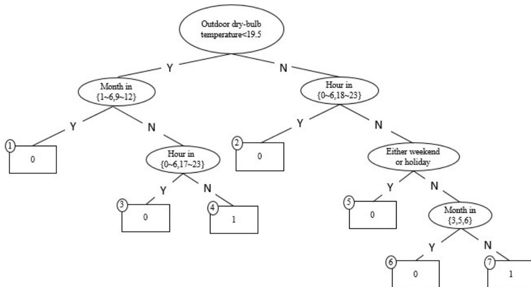
**Figure 1.** DT analysis of AC operational behavior in Bldg. 5
