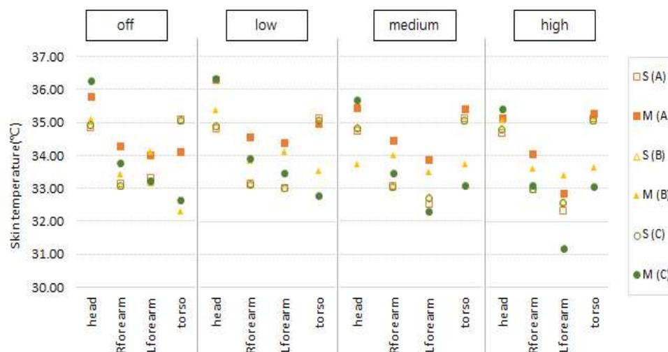
**Figure 2.** Predictions (S) and Measurements (M) of skin temperature by fan mode
