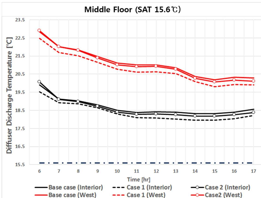
Figure 1. Diffuser discharge temperature for the interior and west zone
