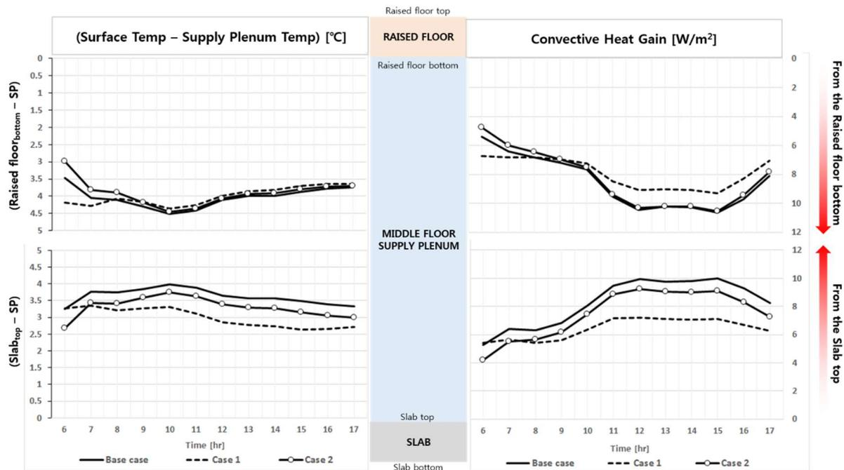
**Figure 4.** Convective heat gain and  $\Delta T$  between surface and plenum in the supply plenum (middle floor, interior, SP = supply plenum)
