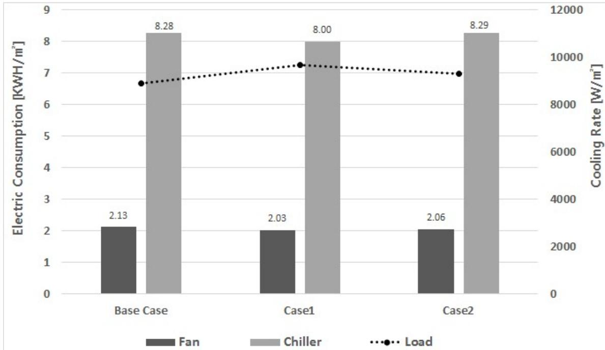
*Figure 5. Cooling load for the interior zone and electric energy consumption*
