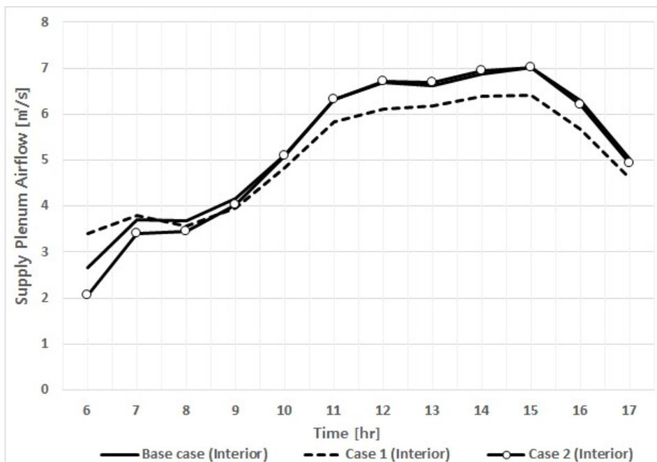
Figure 3. Supply airflow rate for the supply plenum (middle floor, interior)
