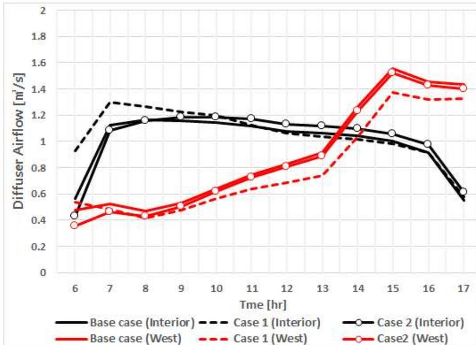
Figure 2. Supply airflow rate for the interior and west zone
