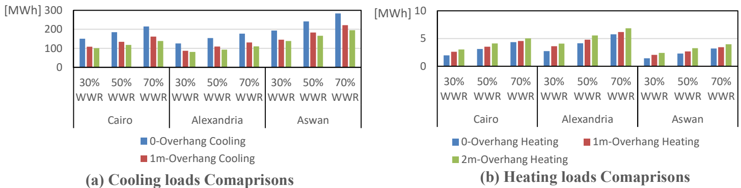
Fig. 5. Effect of WWR on Thermal Loads.
