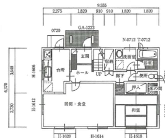
**Figure.1** The 1<sup>st</sup> floor plan of model house (IBEC, 2002)
