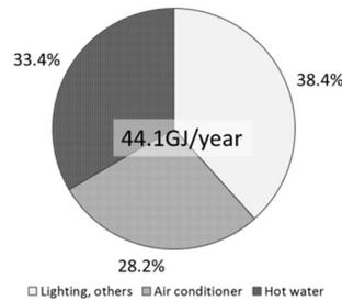
**Figure2.** Breakdown of annual primary energy consumption
