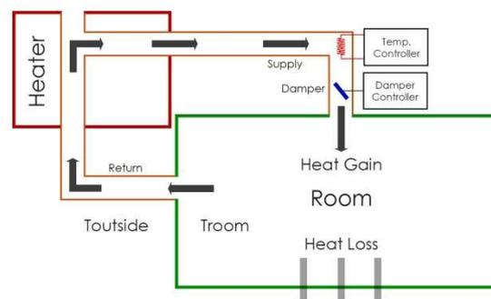
*Figure 1 Diagrammatic flow of HVAC model*
