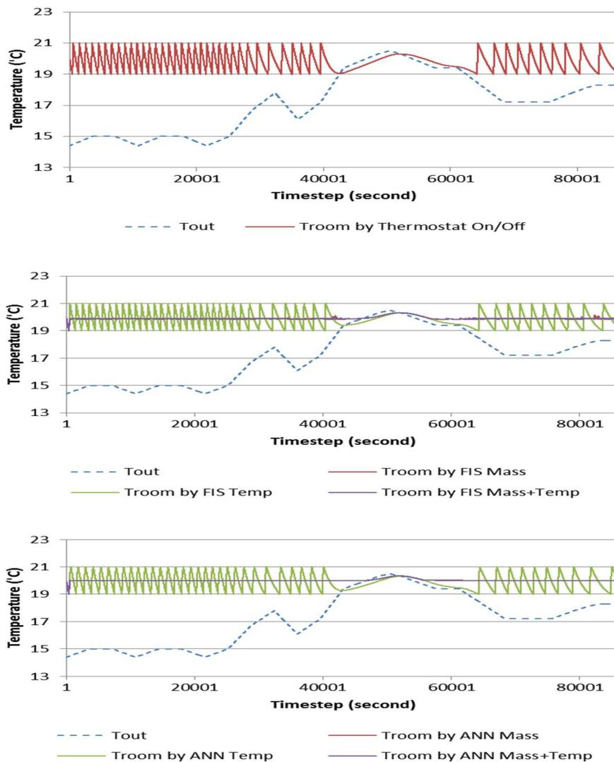
**Figure 4** Outdoor Temperature ( $T_{out}$ ) vs. Room Temperature ( $T_{room}$ ) by 7 controllers
