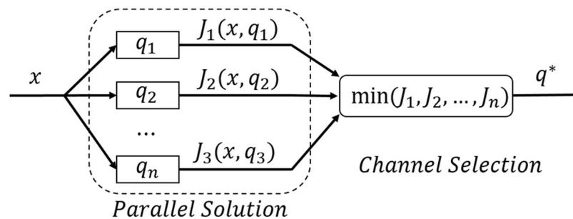
**Figure 2.** Parallel MPC operation: selection of the best sub-problem (channel)
