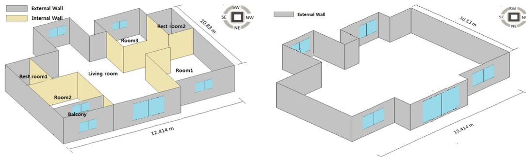
*Figure 1. Differences between multi-zone(left) and single-zone(right)*
