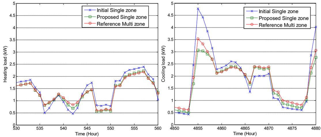
Figure 4. Load comparison: Initial & Proposed single zone, Reference Multi zone
