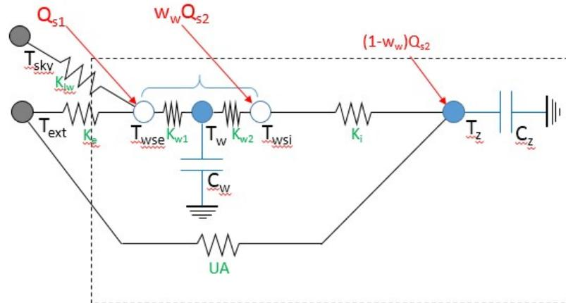
**Figure 3.** Schematic of the RC model (analogy to a 3R2C electric circuit)
