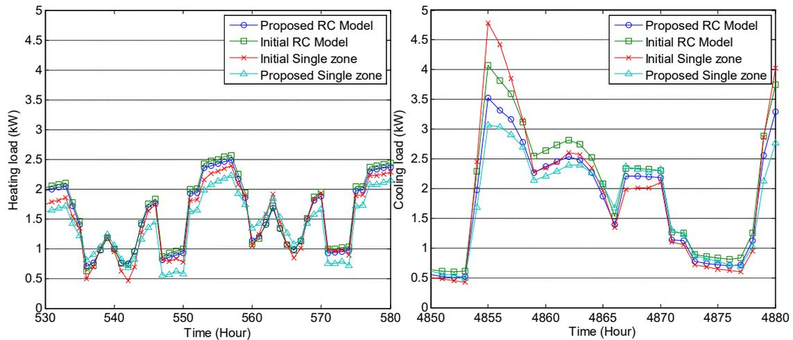
Figure 5. Load comparison: Initial & Proposed RC model and Single zone
