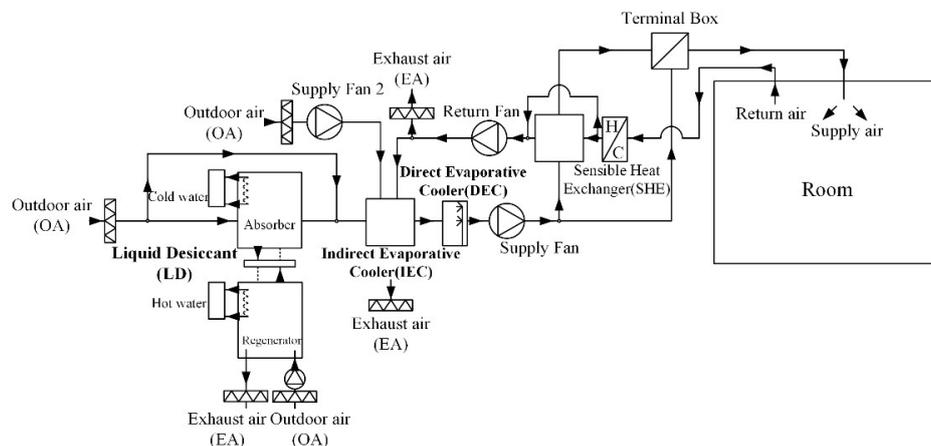
*Figure 1. Schematic diagram of the LD-IDECOAS*
