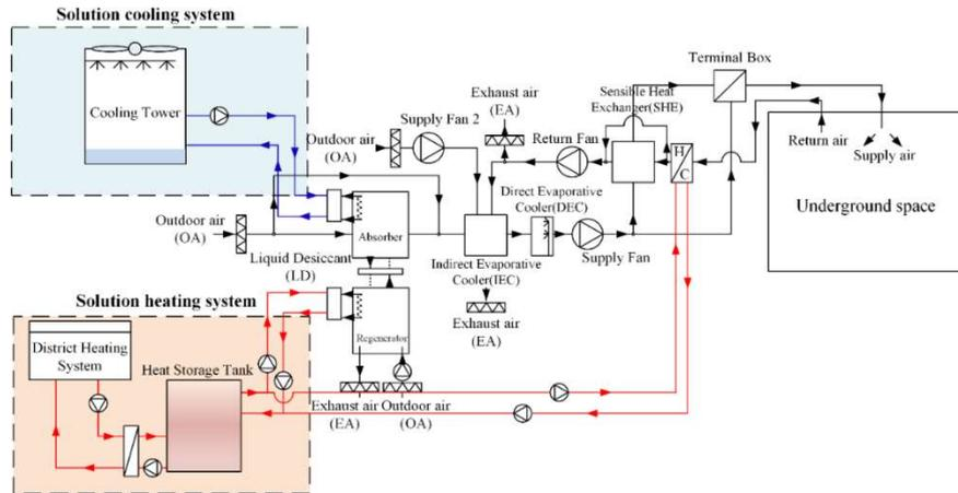
Figure 4. The schematic of the LD-IDECOAS
