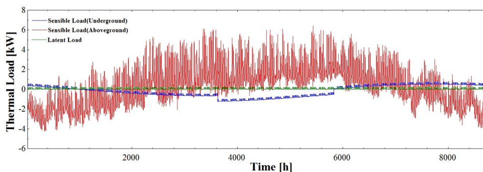
**Figure 3.** Above ground and underground building thermal load behavior
