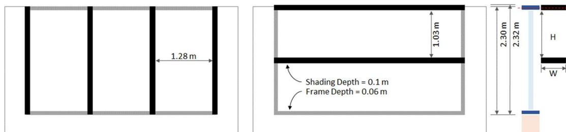
**Figure 2.** Features of shading device cases: (left) Overhang, (right) Fin
