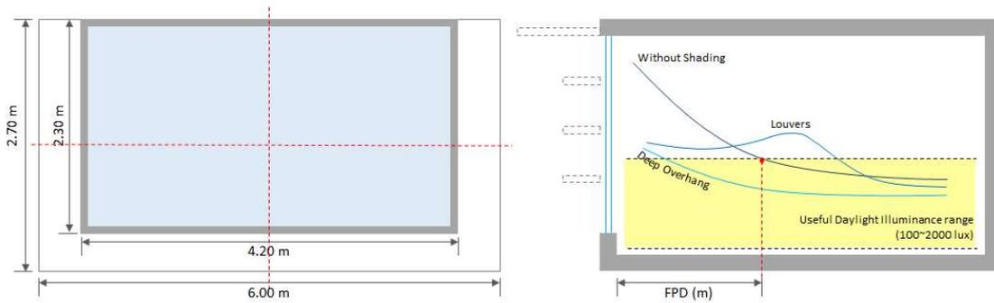
**Figure 1.** Features of the simulation zone(left)&a concept diagram of the FPD(right)
