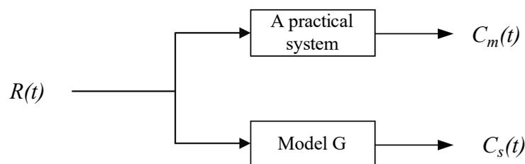
*Fig.1 Identification principle*
