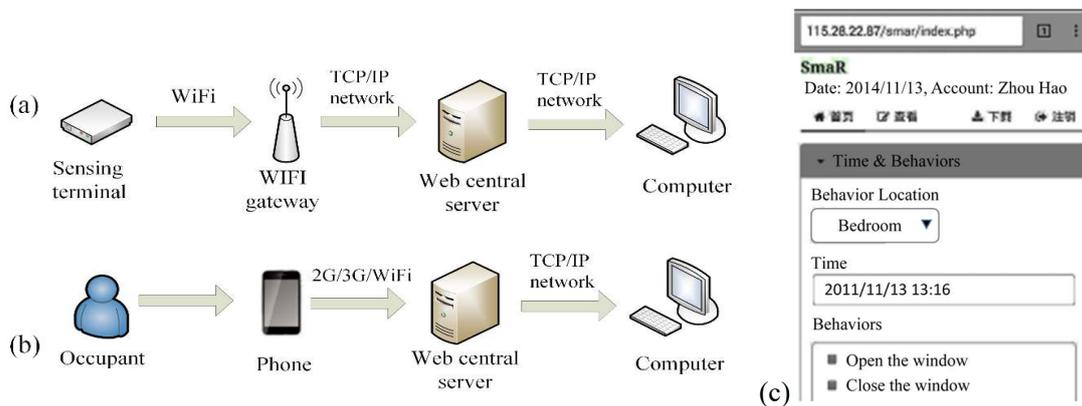
**Figure 1.** Data collection system: (a) environment data, (b) and (c) ground truth data
