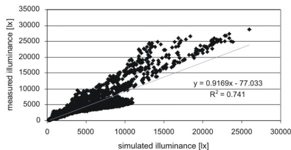
Figure 6 Simulated versus measured indoor illuminance values (sky luminance data based on CIE Standard Skies)
