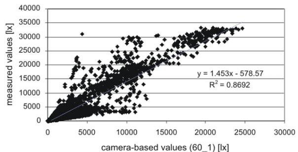
Figure 3 Measured versus calibrated camera-based illuminance values (60\_1)
