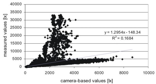
Figure 1 Measured versus initial (non-calibrated) camera-based illuminance values
