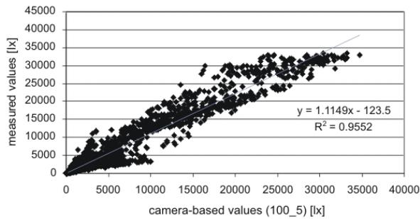
Figure 5 Measured versus calibrated camera-based illuminance values (100\_5)
