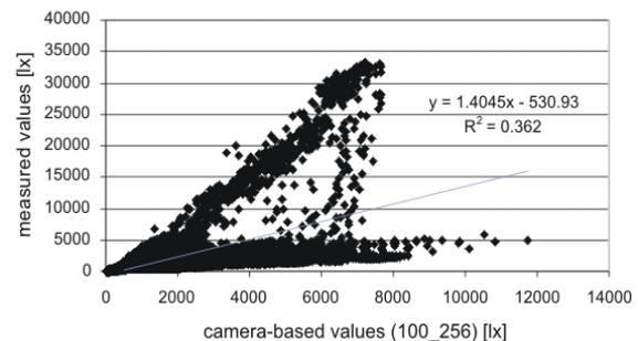
Figure 2 Measured versus calibrated camera-based illuminance values (100\_256)
