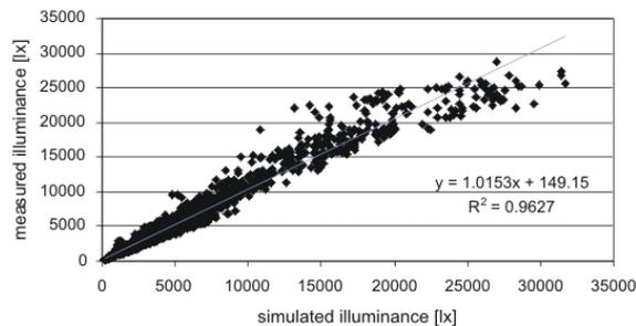
Figure 8 Simulated versus measured indoor illuminance values (sky luminance data based on digital imaging)
