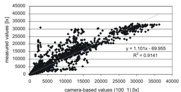
Figure 4 Measured versus calibrated camera-based illuminance values (100\_1)
