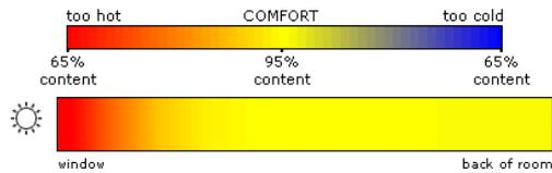
*Figure 3. Thermal comfort during summer. Most occupants feel too hot near the single-pane window.*
