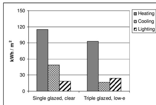
Figure 2. Energy use for two near-identical building designs located in Berlin with different windows.
