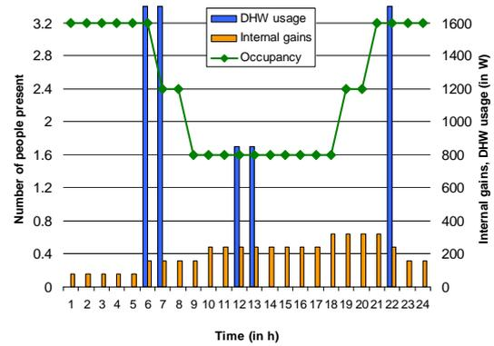
Figure 6: Daily profile of occupancy, internal electricity gains and DHW usage
