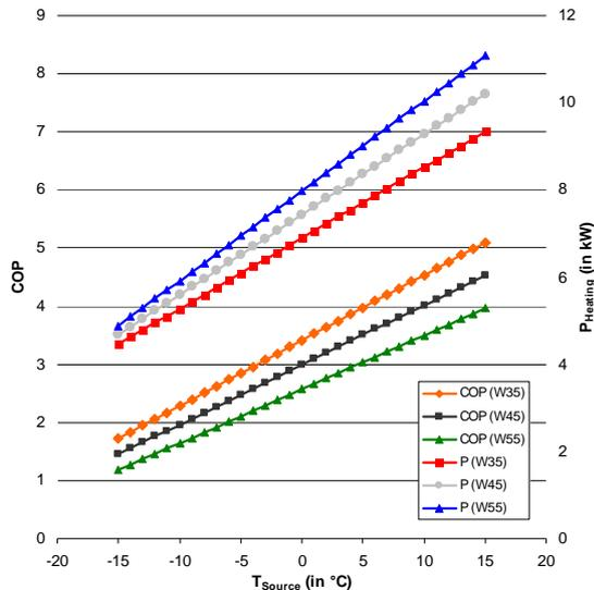
Figure 8: Heat pump characteristics
