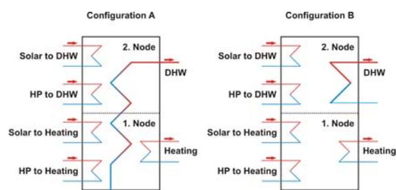
Figure 11: Tank storage configurations
