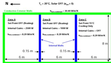
Figure 2: Case MZ320 3-Zone Steady-State Conduction Analytical Verification Test
