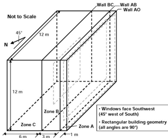
Figure 4: Case MZ360 In-Depth Internal Window Calorimeter
