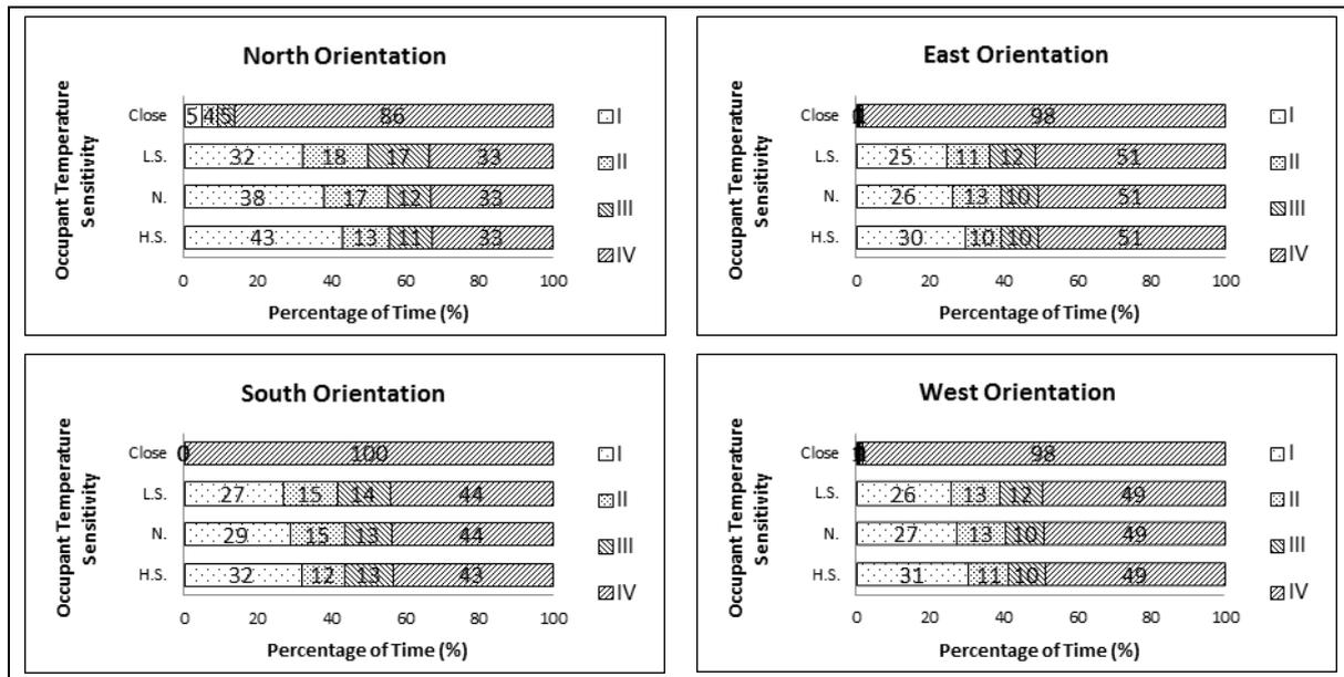
Figure 3: Time percentage of different categories of thermal comfort during the cooling period in the test room for various types of occupant temperature sensitivity (DEC: OFF, Window: Adjustable or Close)
