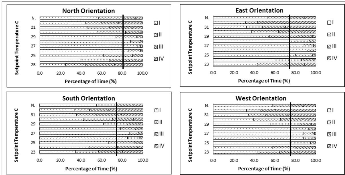
Figure 7: Time percentage of different categories of thermal comfort during the cooling period in the test room for a manually and thermostat controlled DEC (Window: Adjustable, People thermal sensitivity group: Normal Sensitivity)
