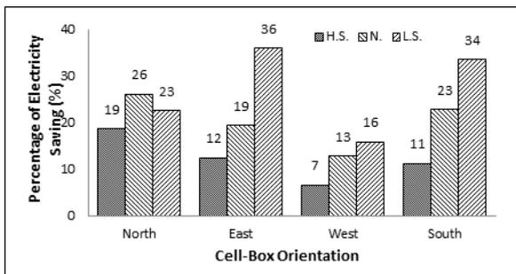
Figure 5: Percentage of decrease in the electricity consumption of DEC due to benefitting from natural cooling ventilation for various types of occupant temperature sensitivity in four orientations of test room (DEC: Manual control, Window: Adjustable)
