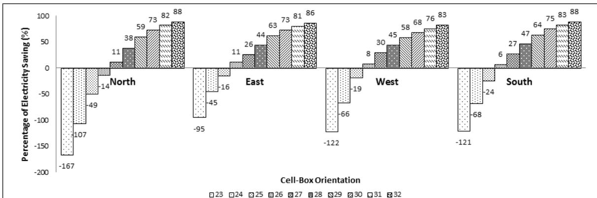
Figure 6: Percentage of decrease in the total electricity consumption of a DEC due to using a thermostat in different setpoint temperature, for four orientations of test room (Window: Adjustable, People thermal sensitivity group: Normal Sensitivity)
