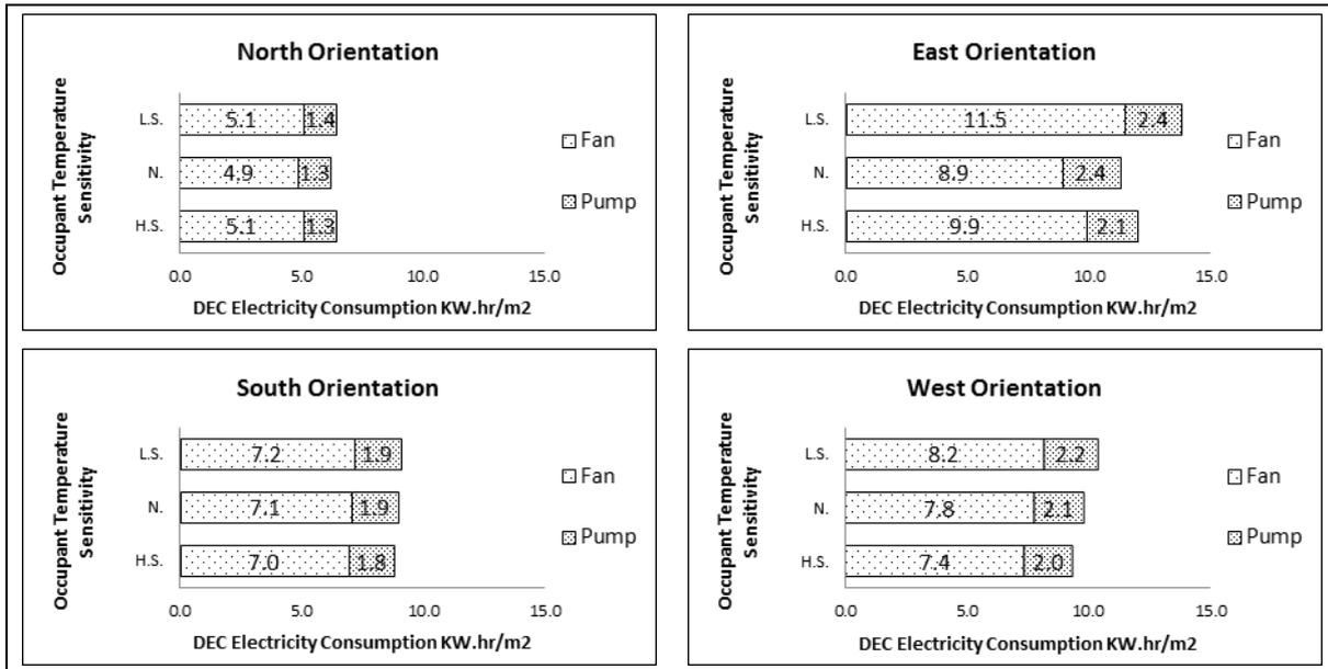
Figure 4: Electricity consumption of DEC during cooling period for various types of occupant's temperature sensitivity (DEC: Manual control, Window: Close)
