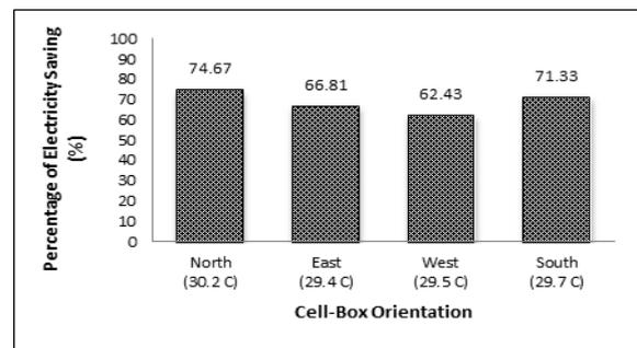
Figure 8: Percentage of decrease in the total electricity consumption of a DEC due to use of a thermostat in the setpoint temperatures that creates similar thermal comfort as a manually controlled DEC, for four orientations of test room (Window: Adjustable, People thermal sensitivity group: Normal Sensitivity)
