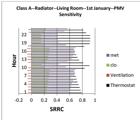
Figure 6: Class A—Radiator—Living Room—PMV sensitivity for January
