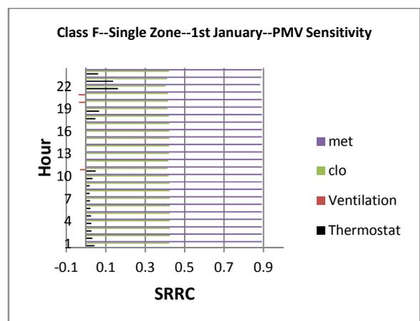
Figure 3: Class F—Single Zone—Ideal Loads—PMV sensitivity per hour for the first day of January
