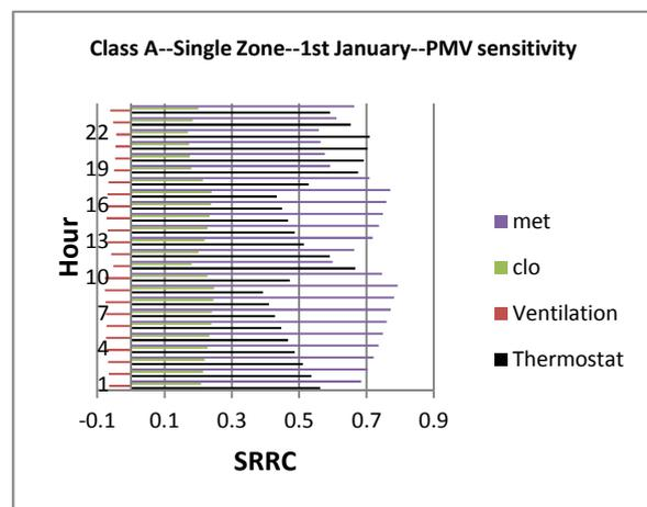
Figure 2: Class A—Single Zone—Ideal Loads—PMV sensitivity per hour for the first day of January
