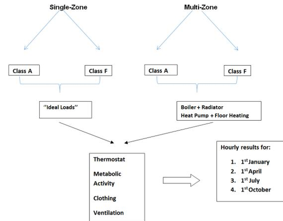
Figure 1: Schematic representation of simulations and combinations between buildings types and parameters
