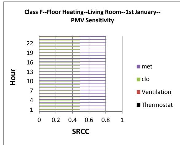
Figure 8: Class F—Floor Heating—Living Room—PMV sensitivity for January
