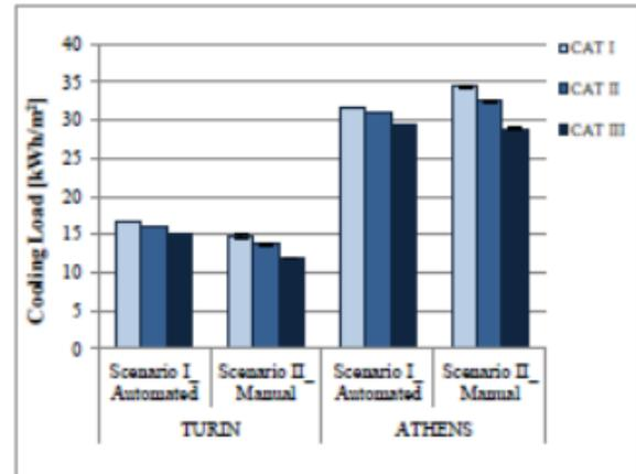
Figure 3: Simulated annual cooling loads in the office reference building located in Turin and Athens
