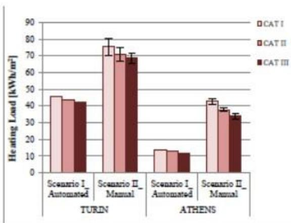
Figure 2: Simulated annual heating loads in the office reference building located in Turin and Athens
