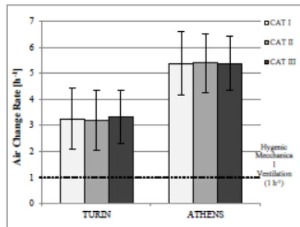
Figure 4: Mean values and standard deviation of air change rates in the office building located in Turin and Athens
