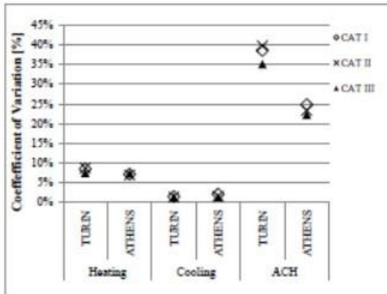
Figure 5: CV values for annual heating, cooling and air change rates
