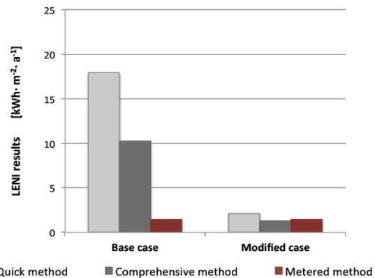
Figure 11: Comparison of LENI-results for Room A for base case and modified case.
