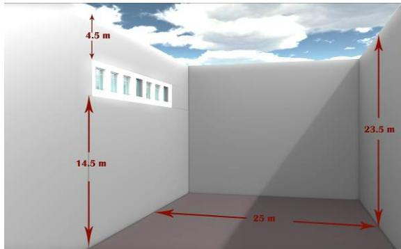
Figure 2: Position of the windows within the building structure and obstructions due to courtyard-perimeter.
