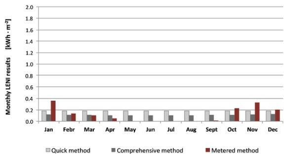
Figure 9: Comparison of the LENI derived from quick method, comprehensive method (modified case conditions) and metered method for room A
