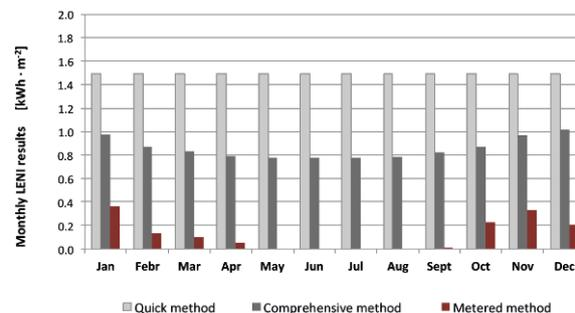
Figure 7: Comparison of the LENI derived from quick method, comprehensive method (base case conditions) and metered method for room A
