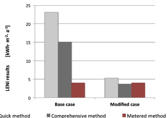
Figure 12: Comparison of LENI-results for Room B for base case and modified case.
