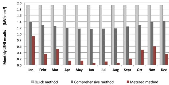
Figure 8: Comparison of the LENI derived from quick method, comprehensive method (base case conditions) and metered method for room B
