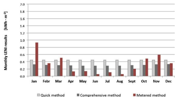
Figure 10: Comparison of the LENI derived from quick method, comprehensive method (modified case conditions) and metered method for room B
