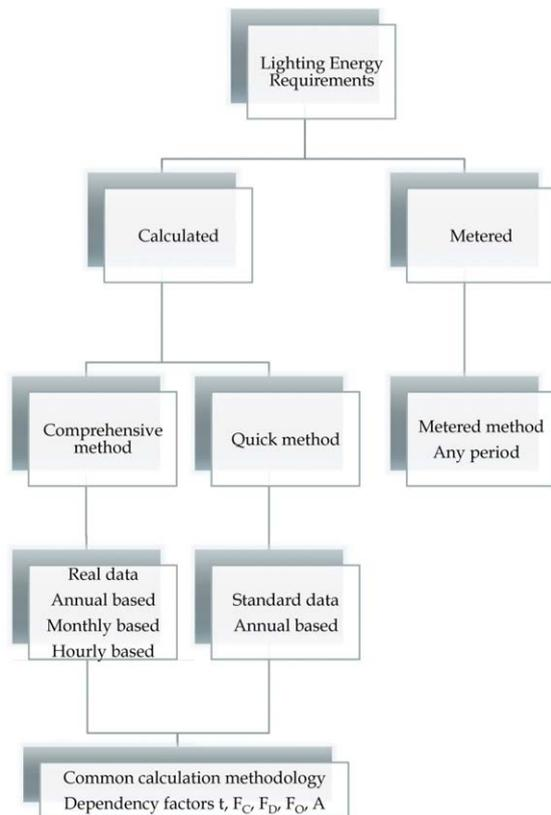
Figure 4: Flow chart illustrating alternative routes to determine lighting energy use (EN 15193 2006)
