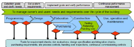
Figure 3. Cx-procedure
