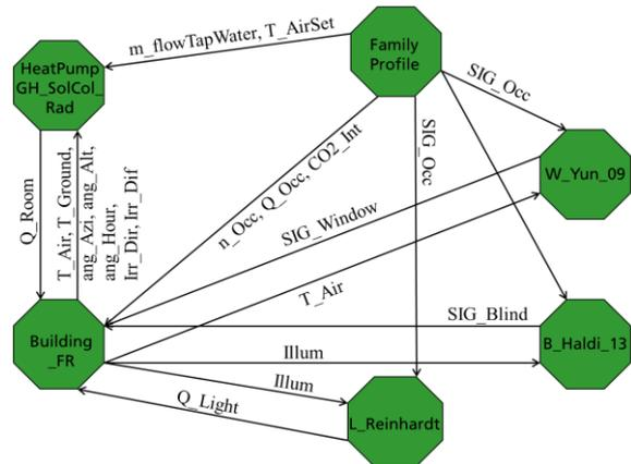
Figure 4: Topology of contributing FMUs in simulation run 4.
