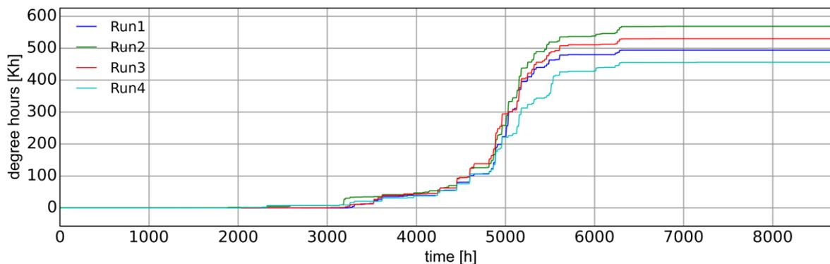
Figure 5: Accumulated degree hours above 26 °C for each simulation run.
