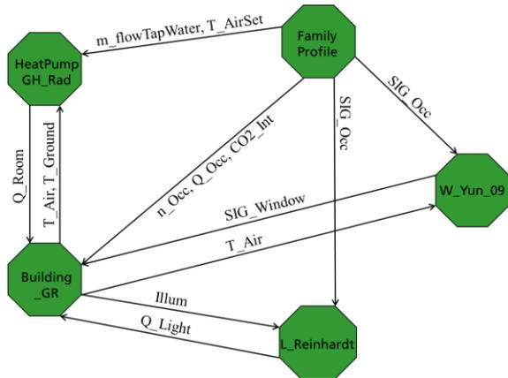
Figure 2: Topology of contributing FMUs in simulation run 1.
