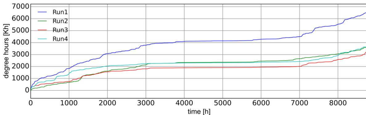
Figure 3: Accumulated degree hours below the temperature setpoint for each simulation run.
