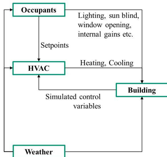
Figure 1: General structure for FMI simulation in BES with main FMU categories framed. Possible exchange variables are noted.
