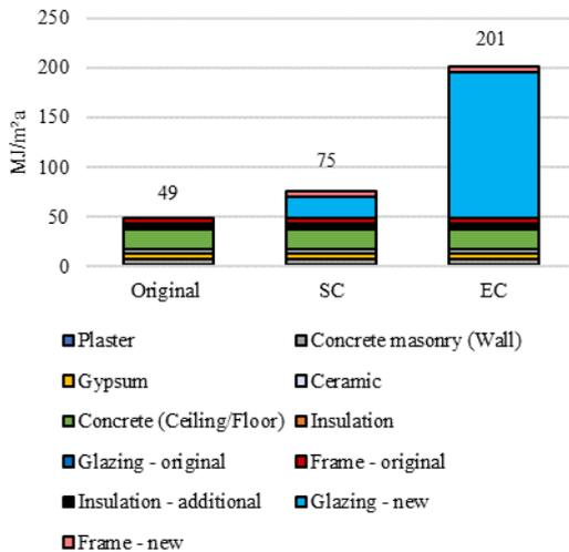
Figure 2: Embodied energy before and after refurbishment
