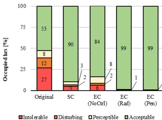
Figure 6: Glare before and after refurbishment
