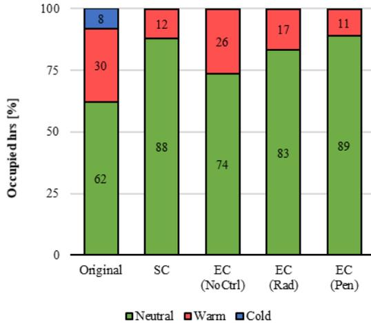
Figure 4: PMV before and after refurbishment
