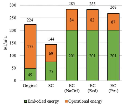
Figure 3: Primary energy before and after refurbishment
