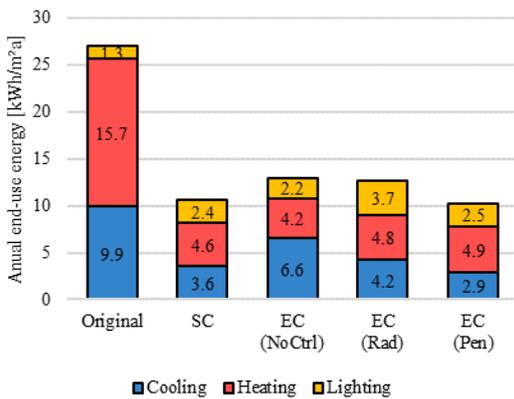
Figure 1: Operational end-use energy before and after refurbishment
