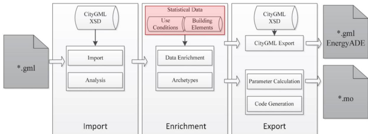
Figure 1: Workflow for an automated building simulation, adapted from (Remmen et al., 2016)
