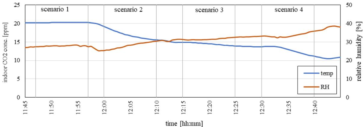
Figure 4: Monitored temperature and relative humidity in the room during the four different scenarios
