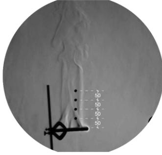
Figure 5 Schlieren visualization of convective thermal plume above hot copper plate and positioning of NTC sensors (black dots, dimension is in mm)
