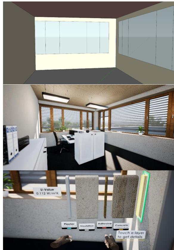
Figure 5: BEM model and VR image corner room with wooden window frames and shading
