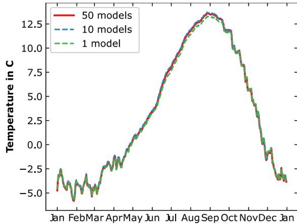
Figure 8: Daily averaged network return temperature at pumping station for different numbers of pipe ground models.
