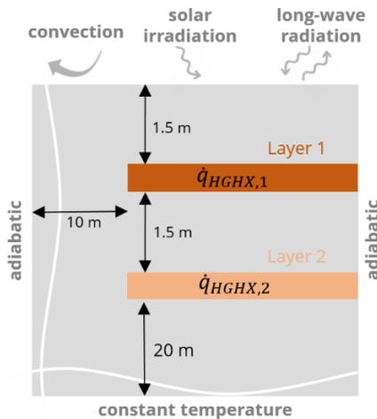
Figure 3: HGHX model geometry and boundary conditions
