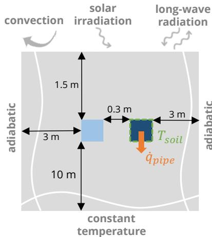
Figure 1: Ground model geometry and boundary conditions
