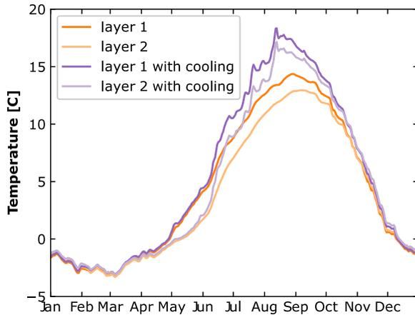
Figure 7: Daily averaged ground temperatures at HGHX layers with and without passive cooling.
