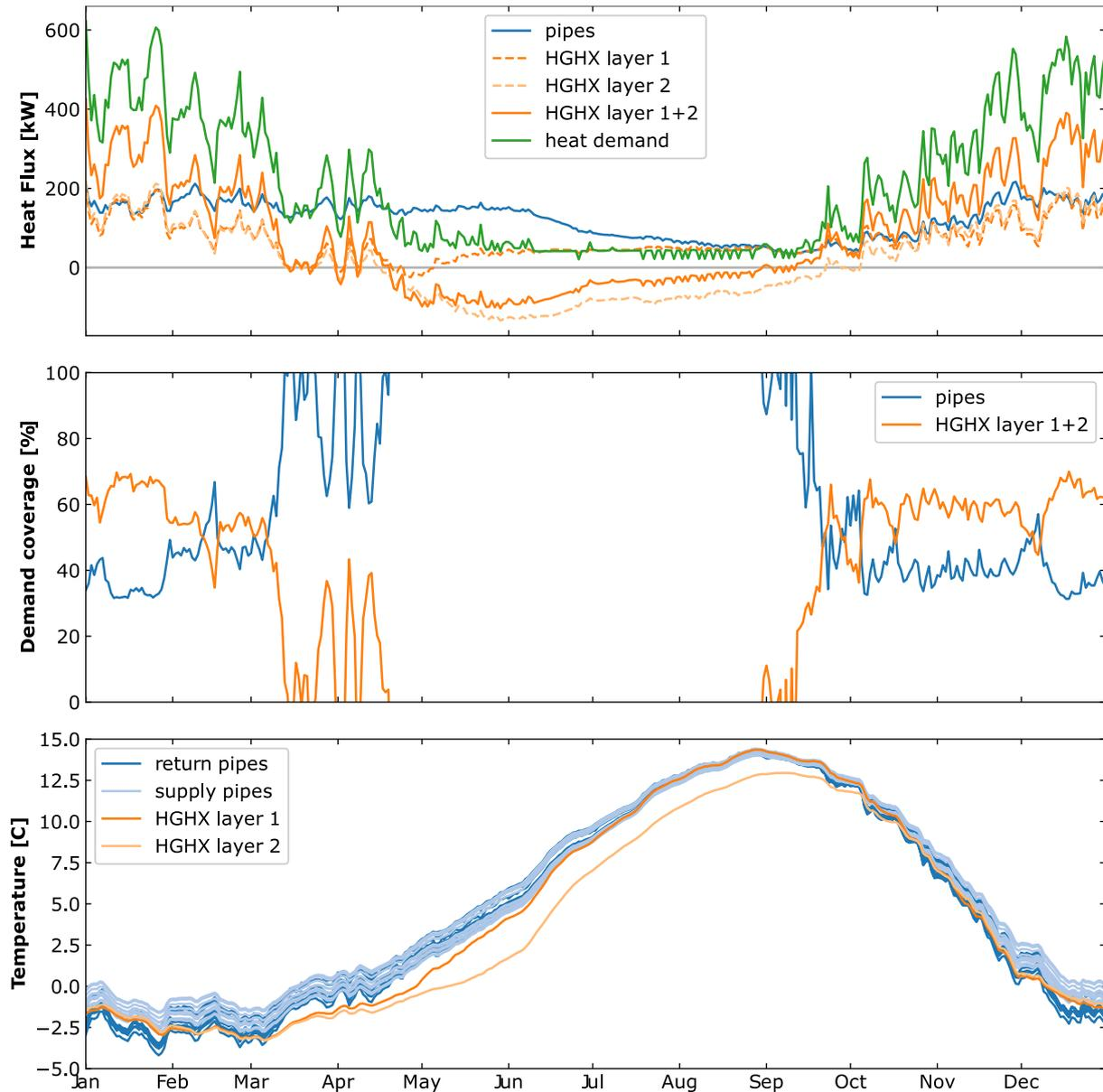
Figure 5: Upper plot: Heat gains from network pipes and HGHX layers. Center plot: Heat demand coverage from network pipes and both HGHX layer. Lower plot: Ground Temperatures at supply pipes (HGHX to buildings) and return pipes (buildings to HGHX) as well as at both HGHX layers. All values are daily averages.
