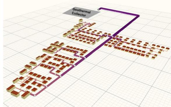
Figure 4: Simulation model of the DHC network in SIM-VICUS. The pipe diameters are scaled by factor 30 for enhanced visibility. Major grid size is 100 m.
