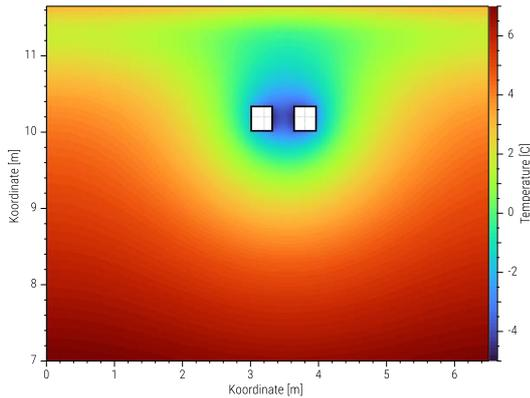
Figure 6: Temperature in ground around pipes at network main supply line at end of February. The pipe diameter is 40 cm.
