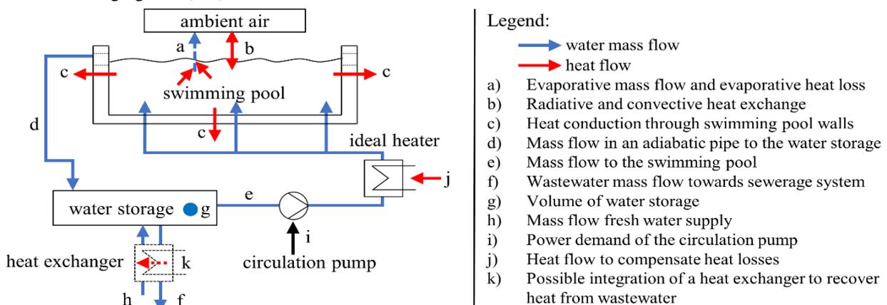
Figure 1: Components, related energy and mass flows within the building model
