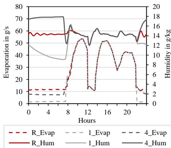
Figure 3: Evaporation of pools and humidity rate in the swimming hall for an exemplary day in May.
