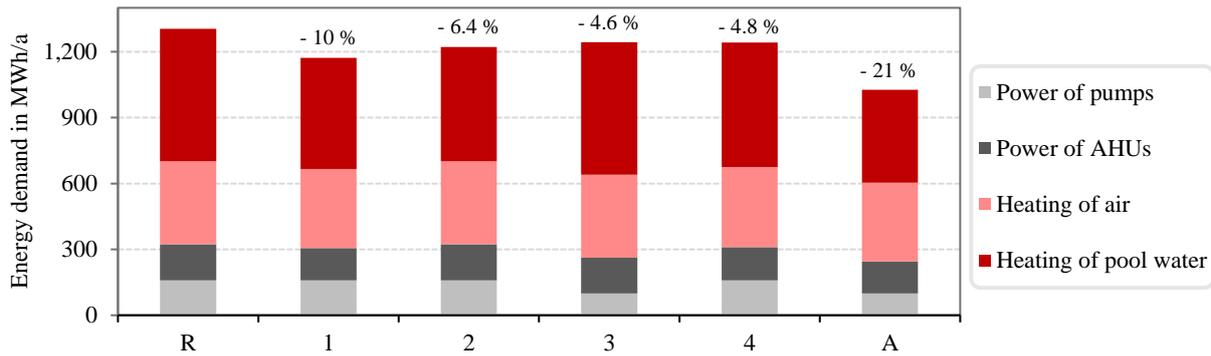
Figure 2: Annual heat and power of the use-case: (R) Reference, (1) Pool cover, (2) Heat recovery, (3) Circulation flow reduction, (4) Increase of humidity, (A) all combined
