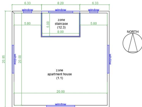
Figure 3. Modeled apartment house with staircase
