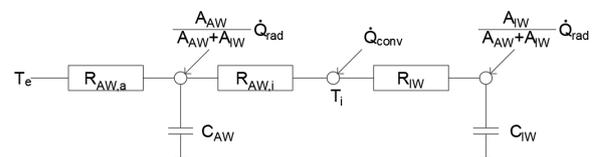
Figure 1. model's equivalent circuit diagram
