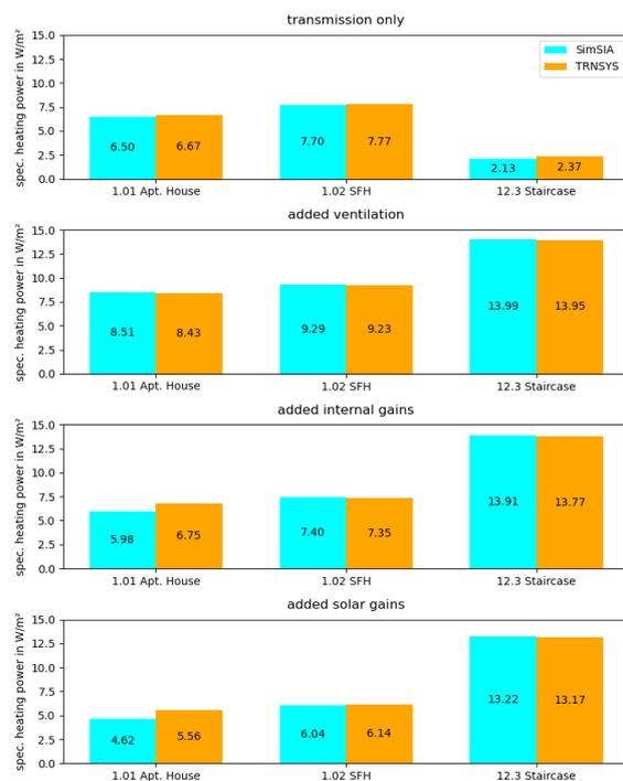
Figure 2. Comparison of steady-state simulation results obtained with SimSIA and with TRNSYS
