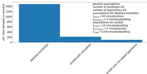
Figure 5. Comparison of processing time between SimSIA and a detailed simulation
