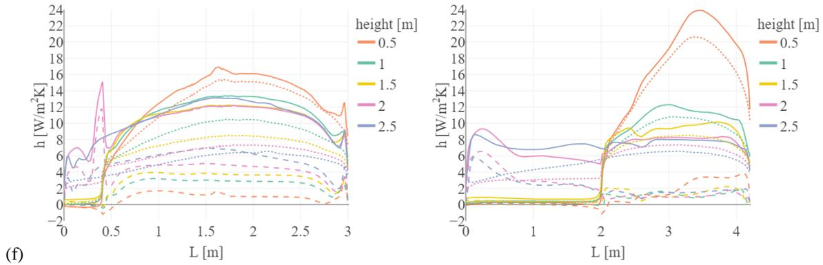
Figure 3:  $h$ ,  $h_{con}$ ,  $h_{rad}$  (solid, dashed, dotted lines) for the exterior walls W1 (left) and W2 (right) as a function of horizontal distance ( $L$ ) from the edge between W1 and W2: (a) C1; (b) C2; (c) C3; (d) C4; (e) C5; (f) C6.
