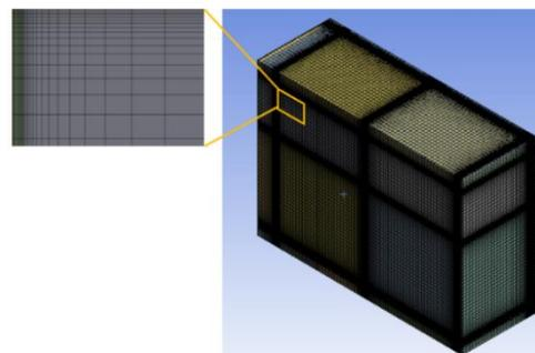
Figure 2: Example of the generated grid near the exterior wall 1 and the ceiling (C2). The figure on the right shows half of the room vertically sliced from the centre of the exterior wall 1.
