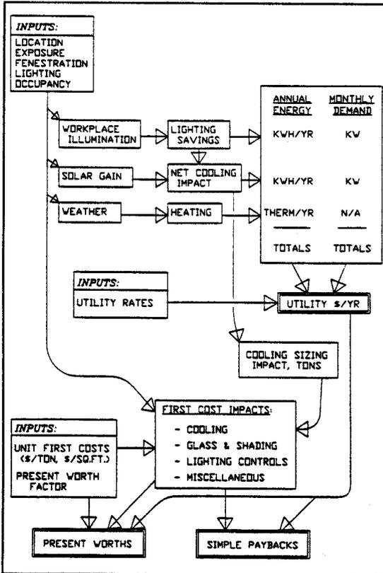
Figure 1. Calculation Structure
