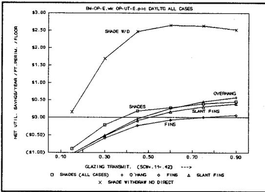
Figure 12. East, Net Utility Savings, Various Shading
