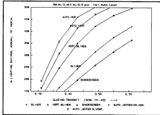
Figure 14. South, Fraction Lighting Saved, Louver Options
