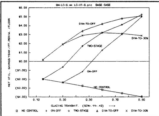
Figure 8. South, Net Utility Savings, Various Lighting Controls
