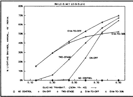
Figure 7. South, Fraction Lighting Saved, Various Lighting Controls
