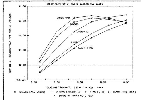
Figure 11. South, Net Utility Savings, Various Shading
